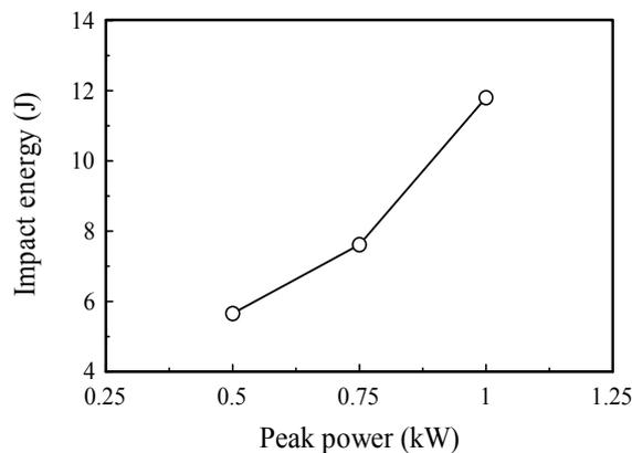
**Figure 5** – Influence of peak power on impact energy;  $f = 50$  Hz and  $P_{av} = 50$  W
