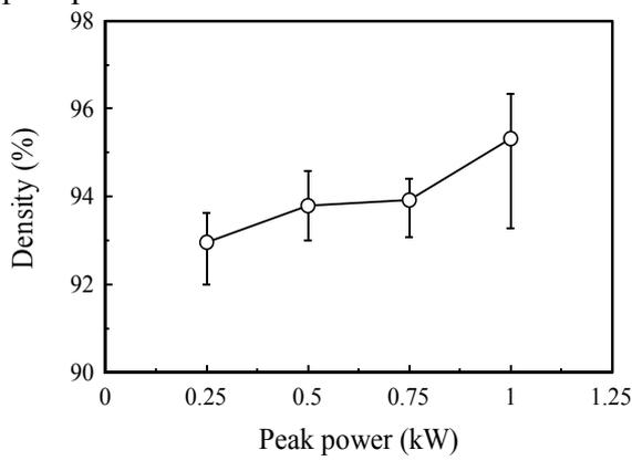
**Figure 3** – Influence of the peak power and scan speed on the density;  $f = 50$  Hz and  $P_{av} = 50$  W
