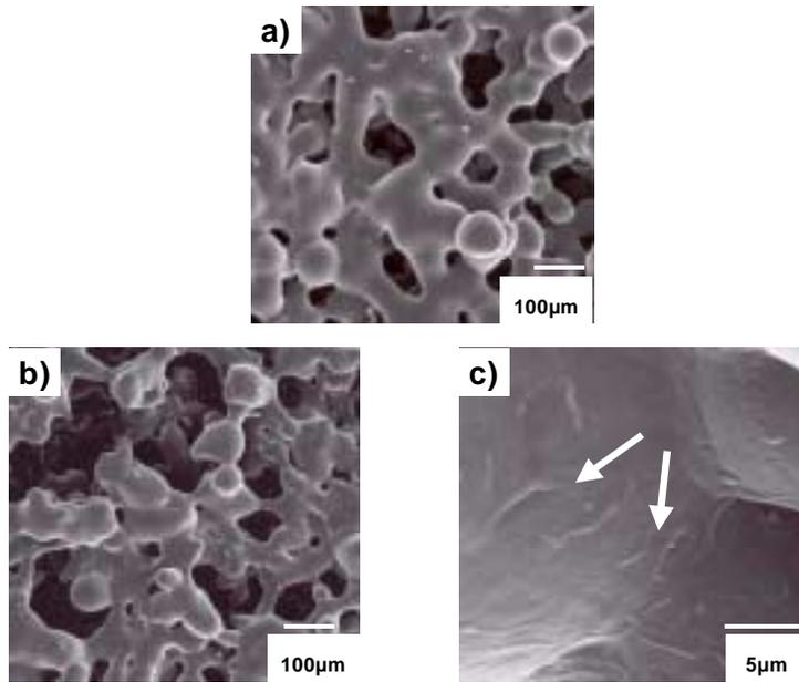
Fig. 4. Sintering result of a) polycarbonate surface morphology (x45) b) nanocomposite surface morphology (x45) and c) morphology near the pore (x2000)
