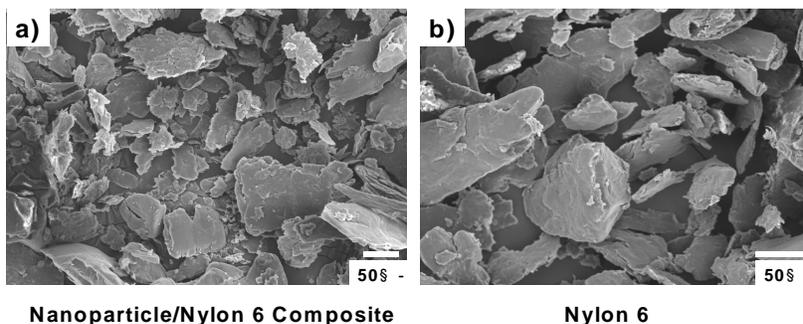
Fig. 2. Powder shape and size distribution of a) Nanocomposite b) Neat nylon 6
