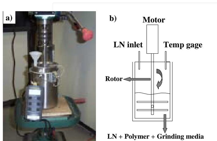
Fig. 1. a) Outer shape of attritor b) Schematic drawing of attritor
