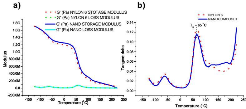
Fig. 3. DMA result of nanocomposite and neat nylon 6
