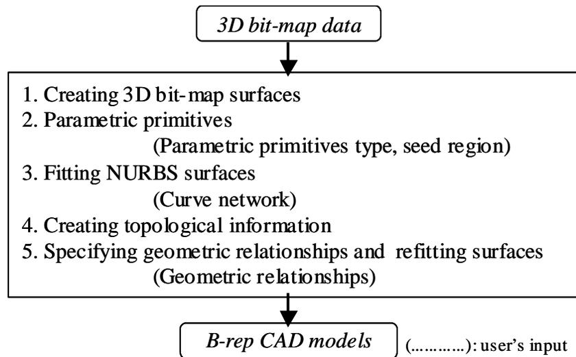
Figure 2. Algorithm for creating B-Rep CAD models
