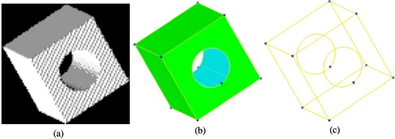
Figure 6. Example of BitCAT applied to 3D bit-map datum
