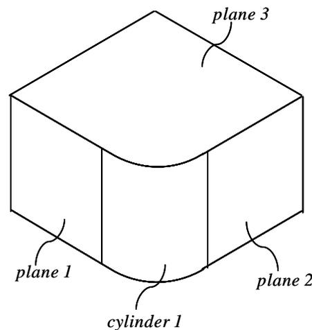
Figure 5. Example of geometric relationships among parametric primitives
