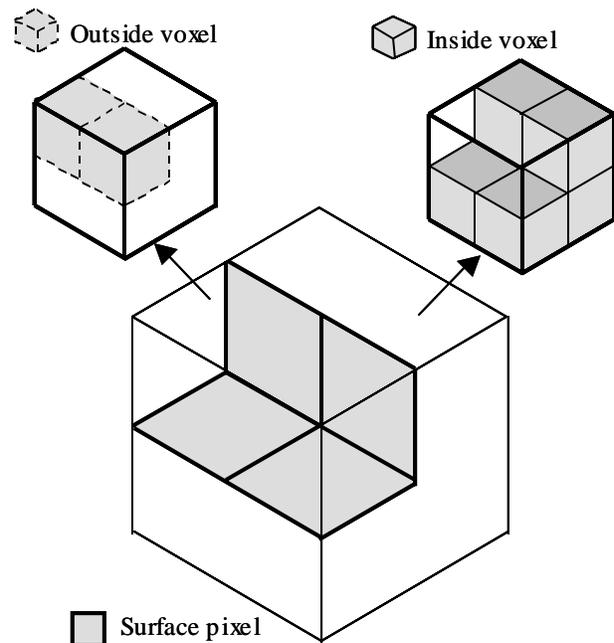
Figure 3. Definition of surface pixels
