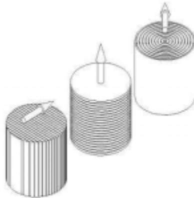
Figure 7. Three basic build directions with a cylinder example
