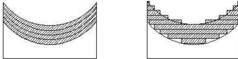
Figure 5. Comparison between conformal layers and planar layers
