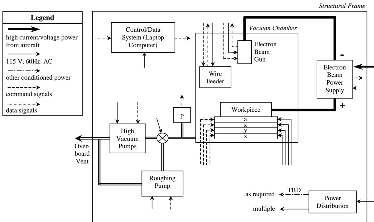
**Figure 2.** Schematic diagram of low-voltage EB F<sup>3</sup> system.
