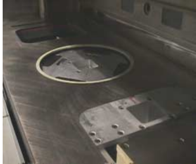
Figure 2. Experimental chamber, single feed with reduced build and feed chamber.
