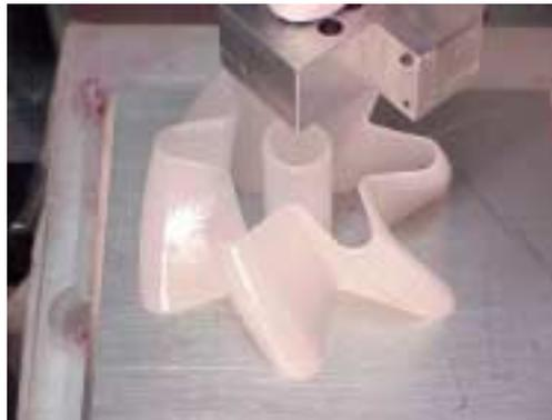
Figure 2: An ice part built by RFP
