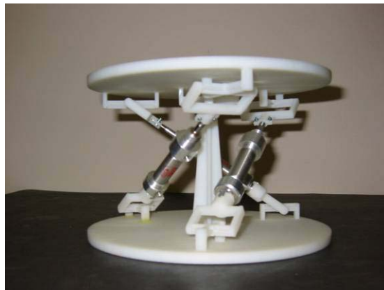
Figure 2: A deposition table constructed using the Compliant Parallel Machine Design Methodology
