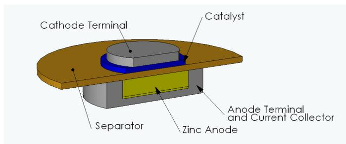
**Figure 6:** Cross-sectional view of freeform fabricated cell design
