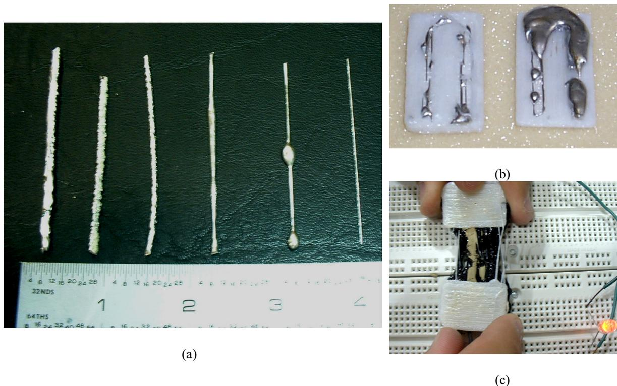
**Figure 10:** (a) Effect of deposition parameters on quality of solder alloy wiring, (b) partial success at embedding solder alloy wiring in thermoplastic part, and (c) flexure joint with silver/methylcellulose paste conductor
