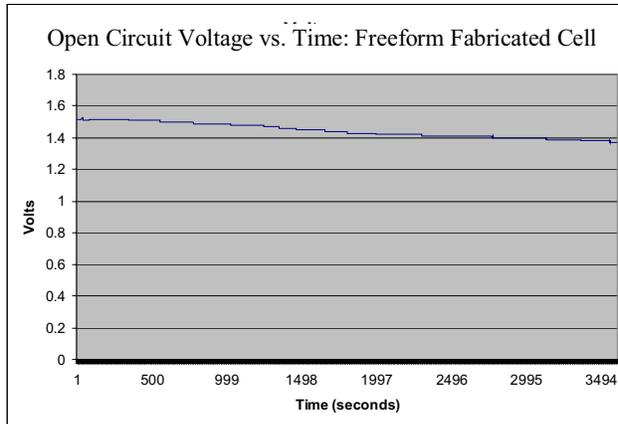
**Figure 8:** Open circuit voltage of freeform fabricated battery
