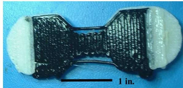
**Figure 9:** ABS and RTV silicone elastomer flexure joint
