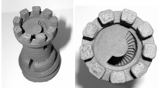
Figure 3. Chess piece built of Ti6Al4V in the EBM S12
