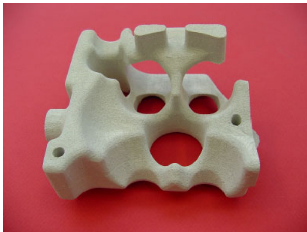
Fig. 5: Laser sintered water jacket core of a single cylinder ( \text{ZrSiO}_4 )
