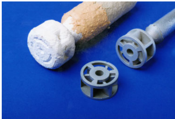
Fig. 3: Impeller wheel cast in AISi7
