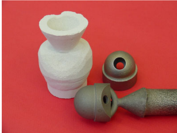
Fig. 4: Whirl chamber of a diesel engine cast in X15CrNiSi25 20
