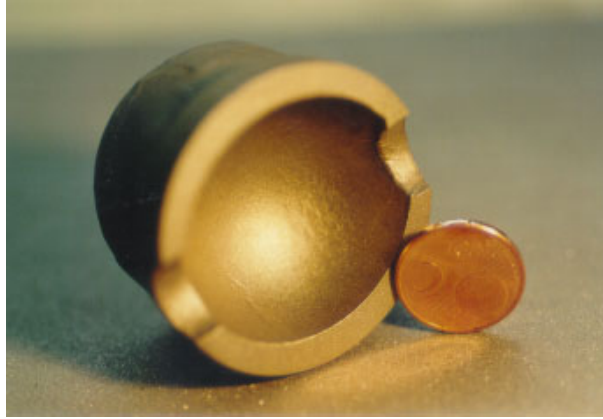
Fig. 6: Cast part split in two with an inner contour made by a laser sintered core
