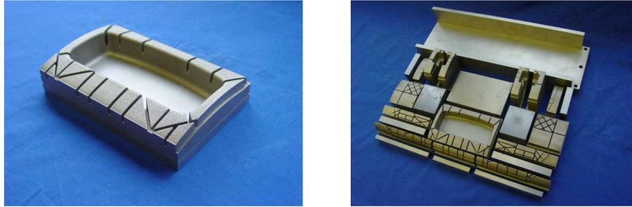
Fig. 9: Laser sintered module (left) and modules of reference tool (right)
