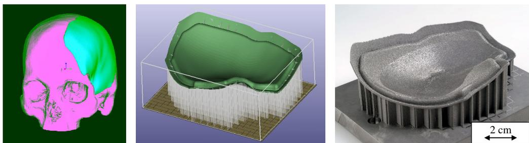
Fig. 4: CAD construction using CT-data (left), data preparation for Laser Melting (middle) and actual Laser Melting part out of Titanium GdII (right)
