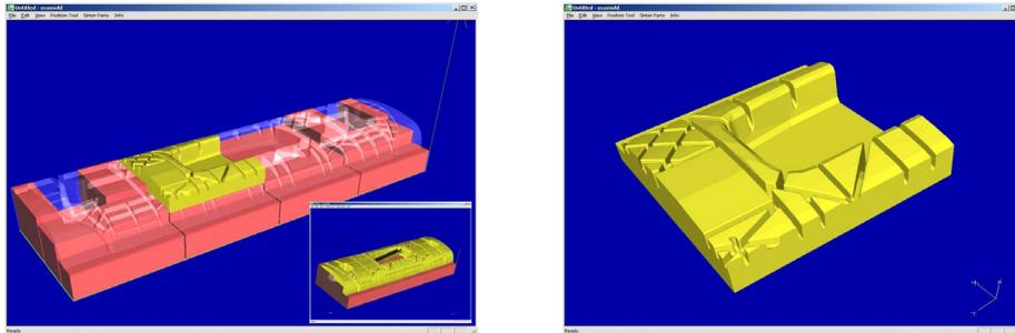
Fig. 7: Automatic calculation of sinter geometry and STL-data of the mold insert
