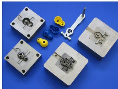
Fig. 15: CMB-made injection molding (left) and die casting (right) inserts together with molded parts
