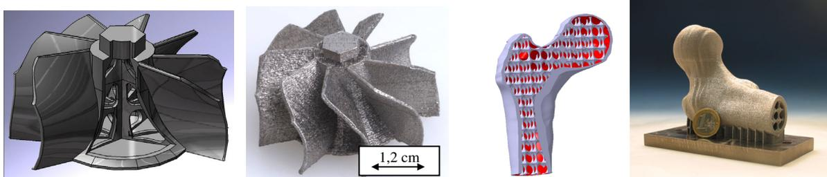
Fig. 5: CAD model and Laser Melting part out of Inconel 718 (left), CAD model and implant with internal structure (right)
