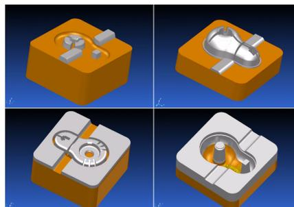
Fig. 14: Die casting (left) and injection molding (right) inserts
