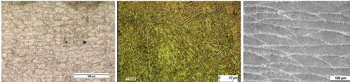
Fig. 1: Cross sections of Laser Melting parts, Tool Steel H13 (left), TiAl6V4 (middle), AlSi10Mg (right)
