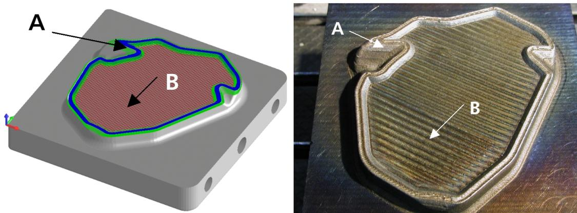
Figure 7: Generation of tools using laser-/ plasma build-up welding
