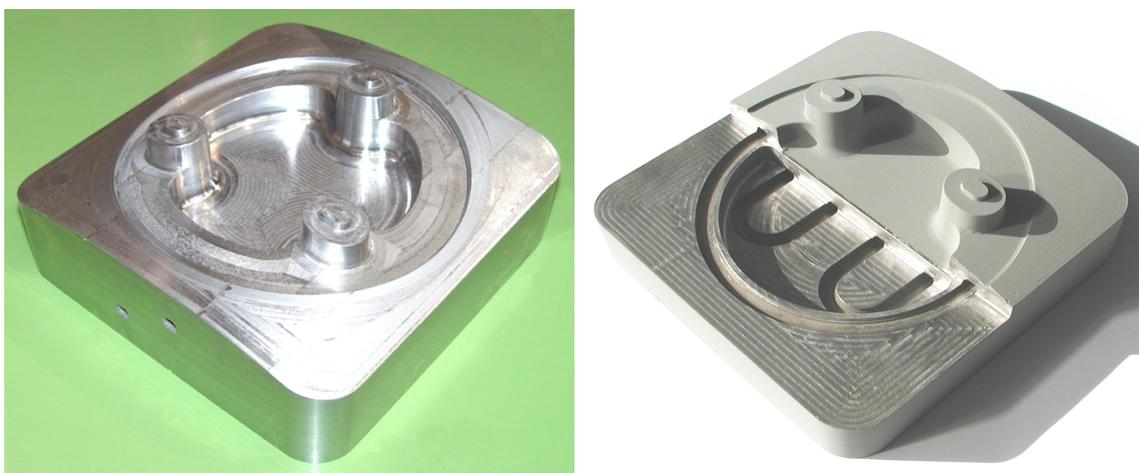
Figure 4: Left finished tool, right: cross sectional view of the cooling system
