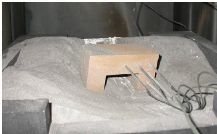
Fig. 3: Test item, thermocouples and test arrangement in the pan covered with aluminum oxide powder.
