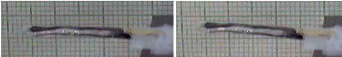
Figure 10. Actuation of silicone encapsulated Nafion/Hydrin; 5V step, elapsed time 50s
