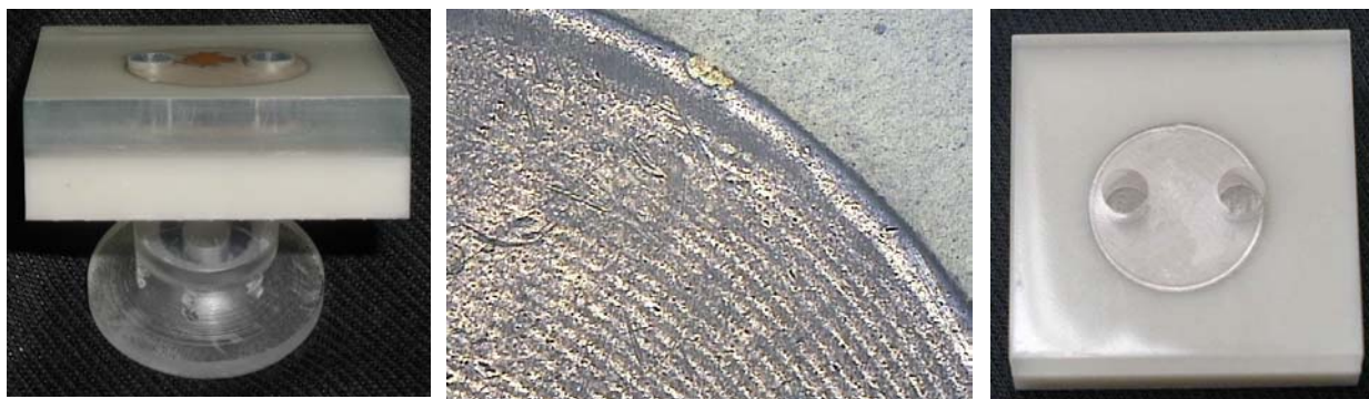
Figure 6. Conductive ink deposited on top of ProtoTool™ base material with a clear WaterShed™ top surface (represents collaborative research with Sandia National Laboratories).
