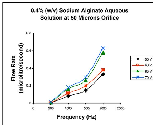
Figure 7: Frequency vs. flow rate for 0.4% (w/v) sodium alginate aqueous solution with 50 microns nozzle diameter using the piezoelectric nozzle system
