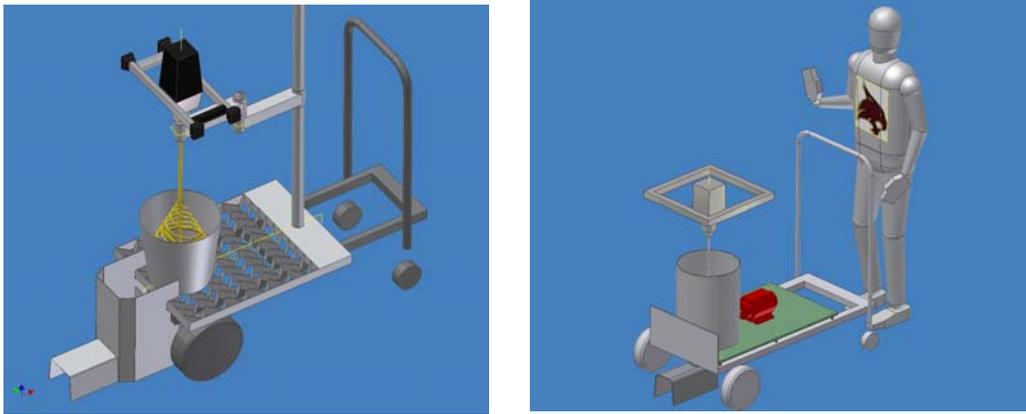
Figure 10: Design I: direct extrusion by centrifuge effect from mixer, Design II: direct extrusion by using vibrator and gravity effect
