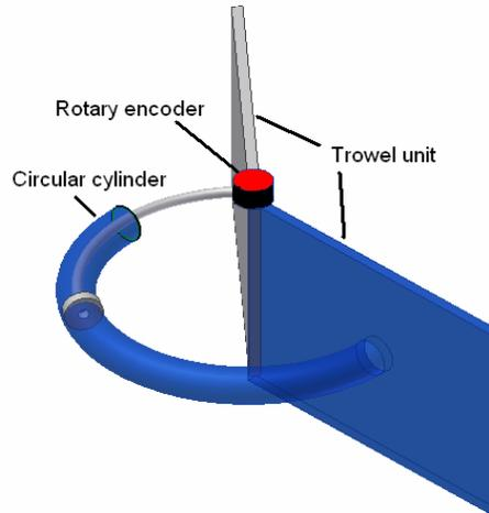
Figure 4: Trowel unit with circular cylinder
