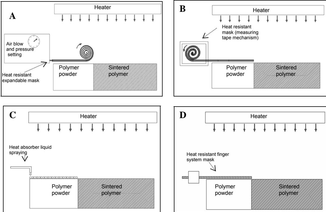
Figure 7. Proposed automated mask systems: A- Air pressure based mask expansion, B- Measuring tape-like expansion mask, C- Heat absorber liquid spraying system, and D- Finger system mask
