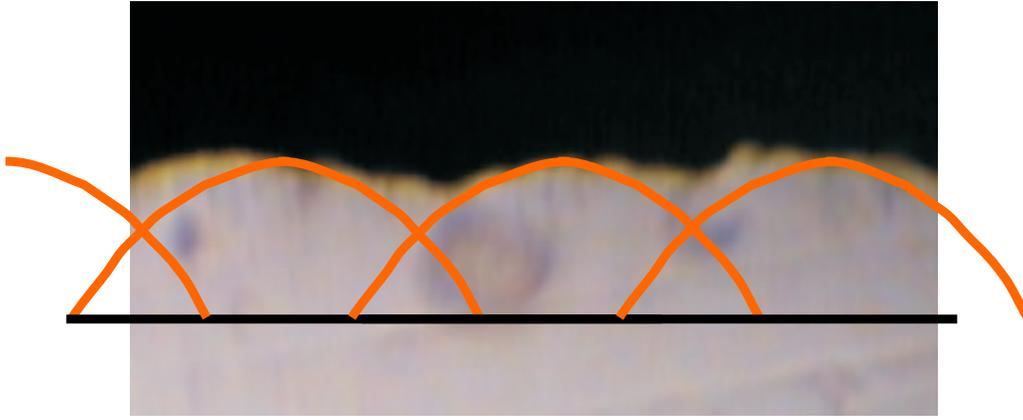
**Fig. 7.** The Cross-sectional profile of the deposited overlapping beads
