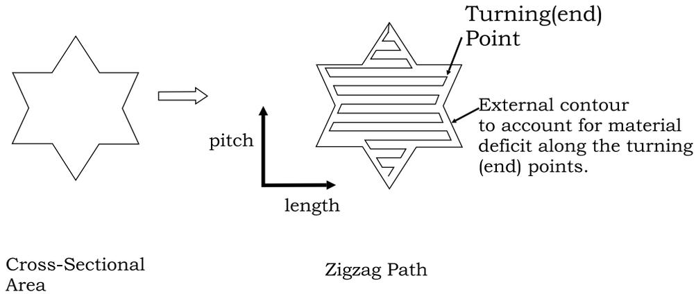
**Fig. 8.** A Cross-sectional area and the corresponding zigzag path
