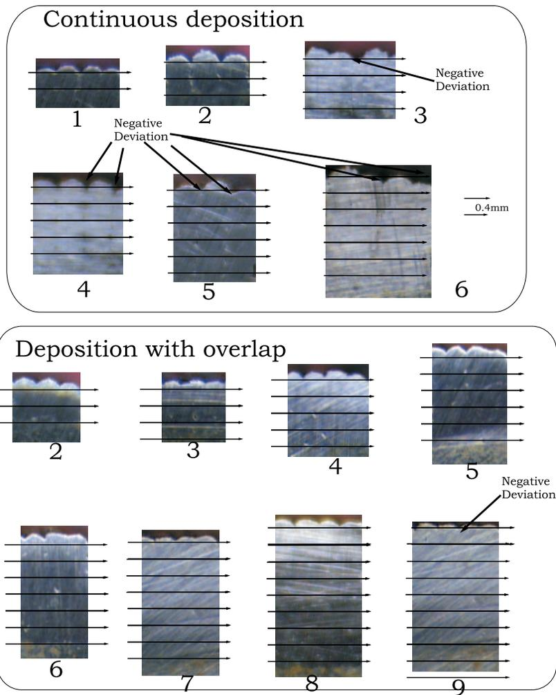
**Fig. 9.** A Cross-sectional view of the beads for different number of layers
