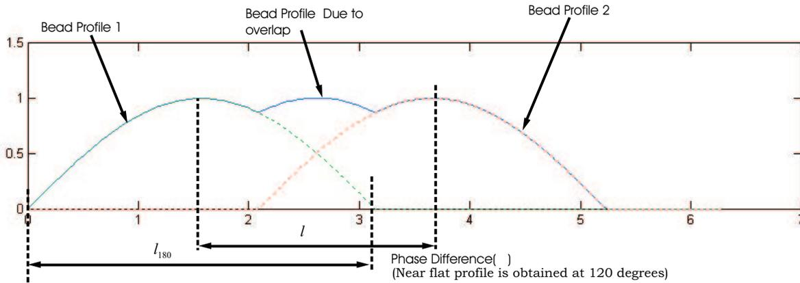
**Fig. 6.** The Optimal Profile Obtained by Overlapping Two Beads
