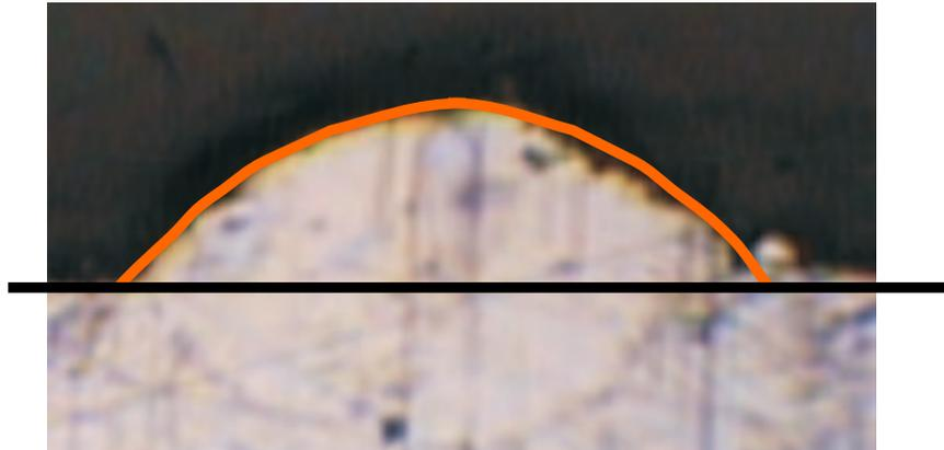
**Fig. 5.** Sinusoidal Approximation of the Bead profile
