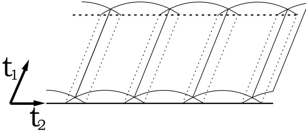
**Fig. 4.** Material deposition defined by the directions  $t_1$  and  $t_2$
