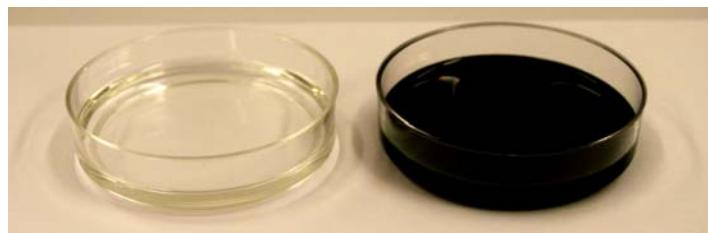
**Figure 3.** Petri dishes containing pure DSM Somos® WaterShed™ 11120 (left) and WaterShed™ 11120 with .05wt% (w/v) of MWCNTs.
