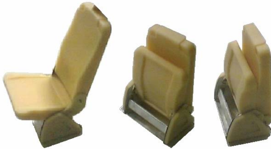
Figure. 6 - SFF hybrid prototype (scale 1:5) made by RP multi-jet in wax reinforced with aluminum at the zones that support rotation axles and on the lower part of the model.
