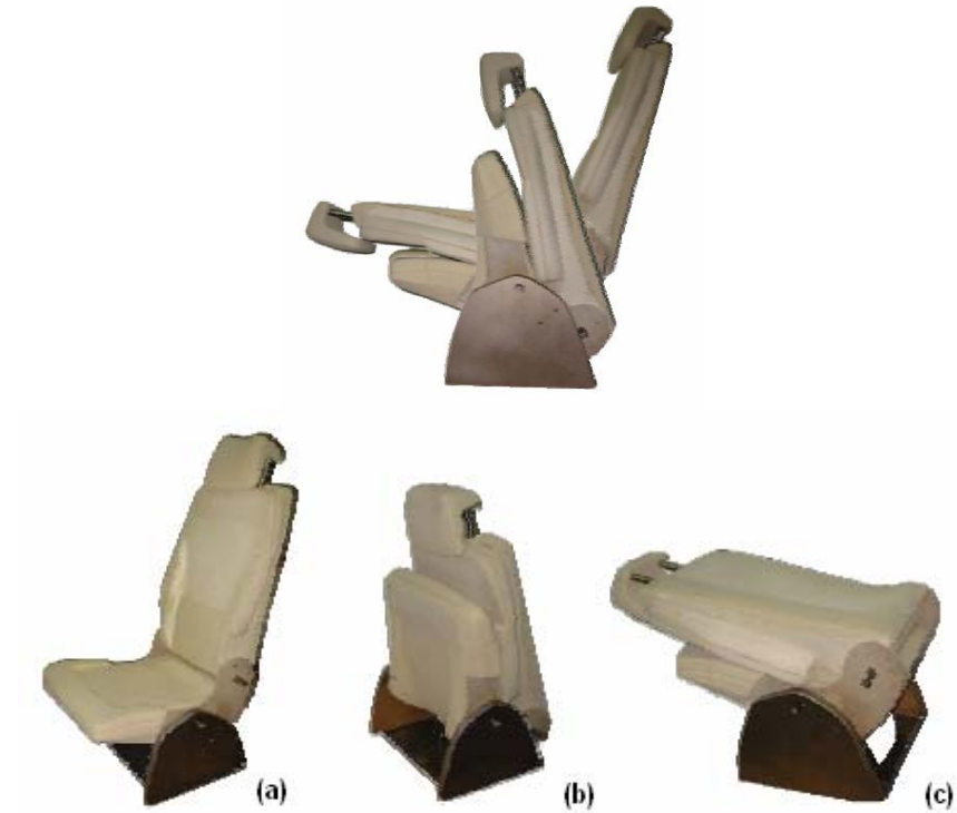
Fig. 7 - The solid freeform hybrid prototype (scale 1:1) performs accurately the main movements of the MPV seat: (a) normal; (b) stored; and (c) table.
