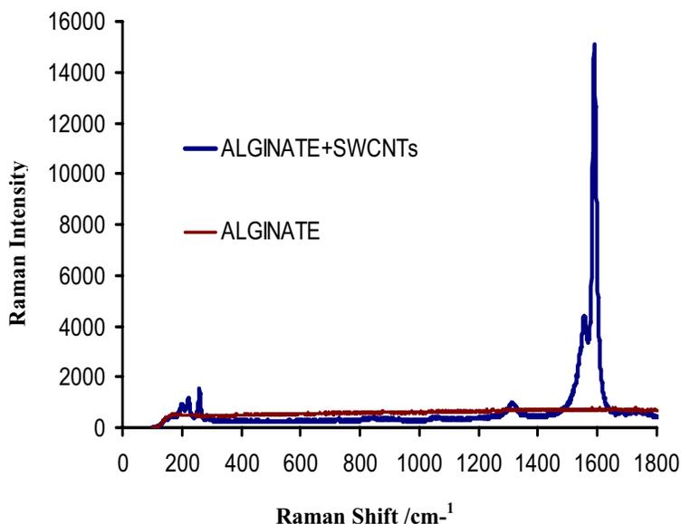
Figure 6: Raman spectrogram of hydrogel scaffolds
