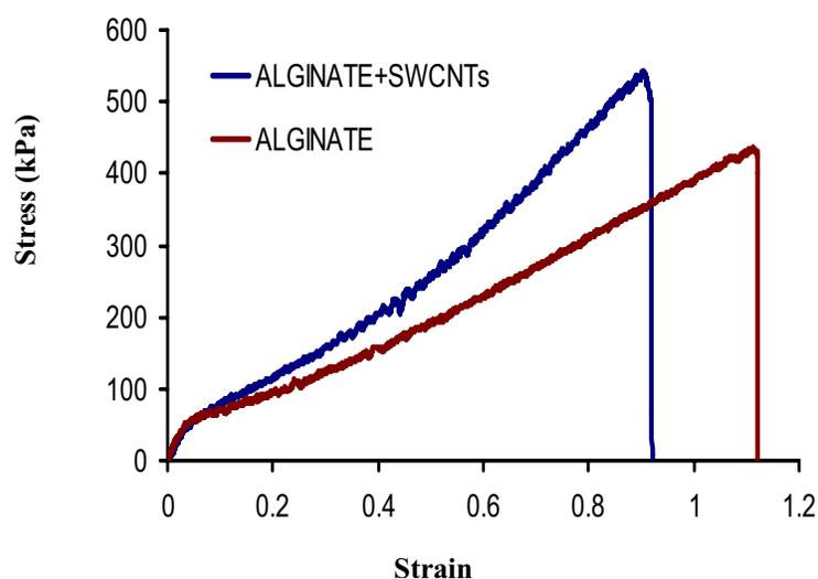
Figure 7: Tensile stress-strain relation of hydrogel strips
