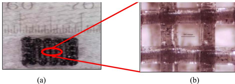
Figure 3: a) Top view of scaffold made with alginate-1% w/w SWCNT-cell mixture
