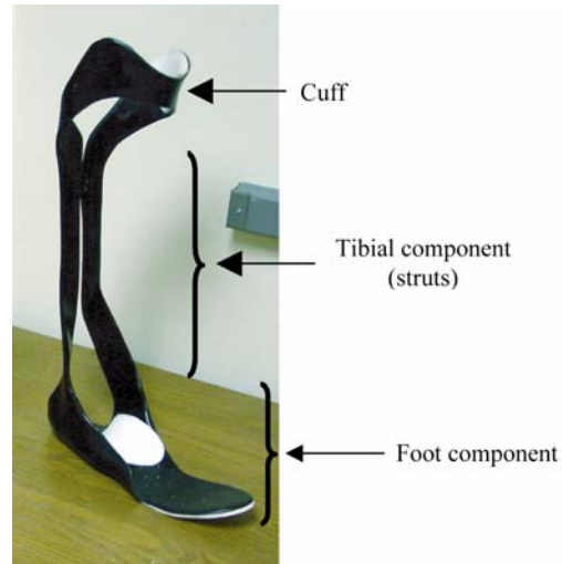
Figure 1: Carbon fiber AFO design (Dynamic Brace, Advanced Prosthetics and Orthotics Inc.)
