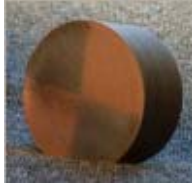
Figure 7: Multi material component made of iron and copper built with the MPP demonstrator.
