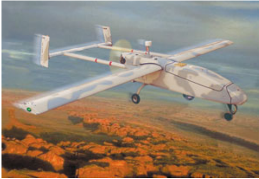
Figure 9. AAI's shadow 400 UAV system [26]
