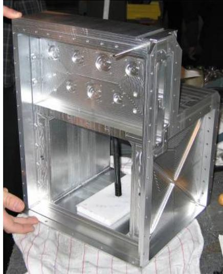
**Figure 1.** Electronics housing showing non-optimized rib-on-plate structure
