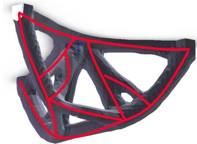
**Figure 6.** The optimized tripod is shown with splines drawn along the legs of the structure.
