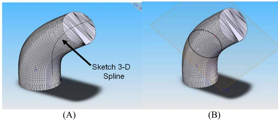
**Figure 7.** For process planning, a spline is drawn along the surface of a part (A) and then planes normal to the spline are constructed(B). The intersection of these planes and the geometry gives a bounding curve used for path planning.
