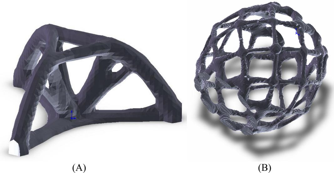
**Figure 3.** Two structures that were optimized using ATO. The tripod structure (A) has 3 simply supported points and a center loading. The loxodrome (B) has high torsional stiffness, but is designed to have bending and axial compliance.
