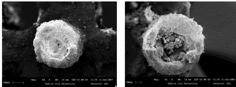
Figure 4 Cross-section of struts fabricated in the Z building direction (a) 0.6 mm, (b) 0.8 mm strut at  $P_{01}=10\text{ W}$
