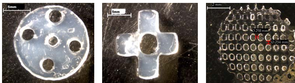
Fig 9. Sample PEGDA samples produced with strand sizes close to 250\mu\text{m} for a 20% PEGDA concentration ratio.
