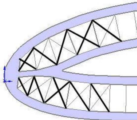
**Figure 11. UAV left section optimization showing retained lattice elements in bold.**
