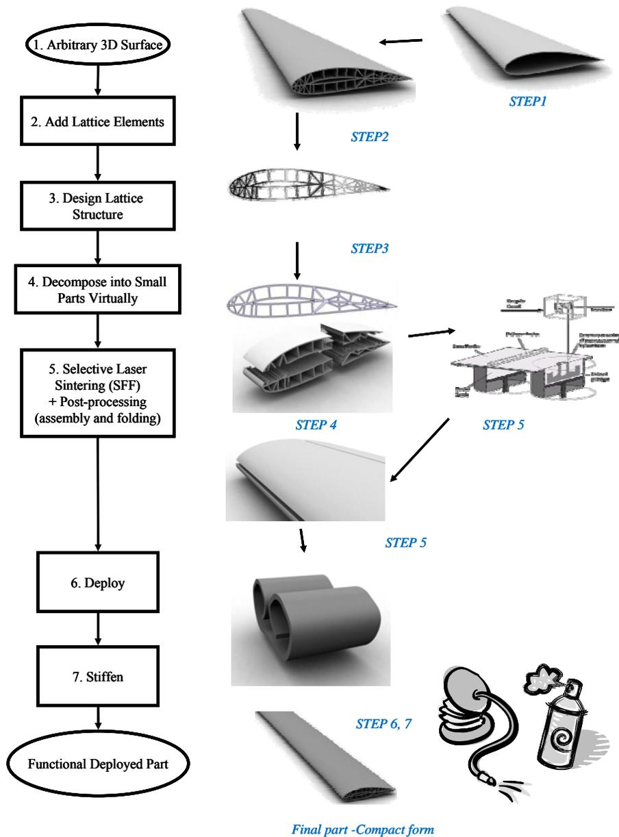
Figure 1. Design methodology for freeform deployable parts with lattice skins.
