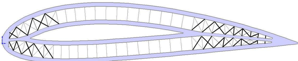
**Figure 15. Final optimal lattice configuration of the UAV wing with retained elements.**
