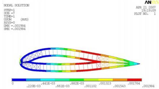
**Figure 12. Deflection result of UAV WING after left section optimization.**
