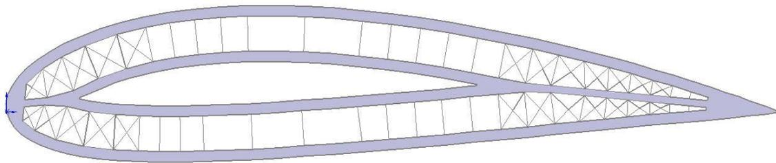
Figure 7. UAV wing profile with initial lattice structure.
