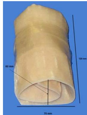
**Figure 19. UAV wing in folded configuration.**
