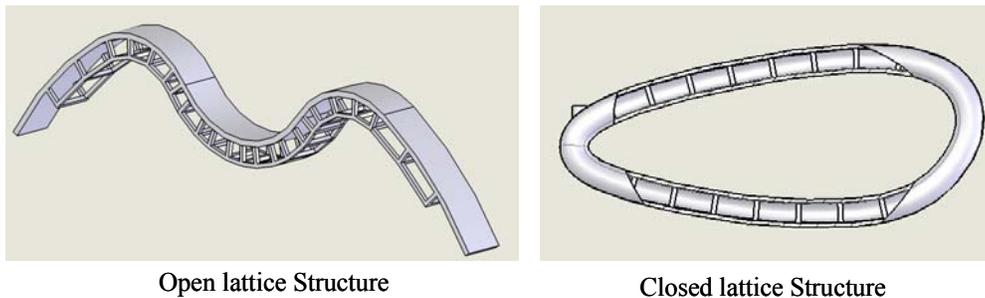
Figure 2. Open and closed lattice structures.
