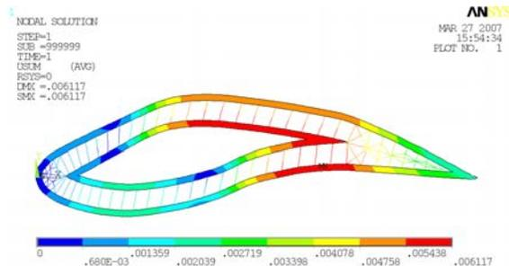
**Figure 10. Deflection of UAV wing profile before optimization**
