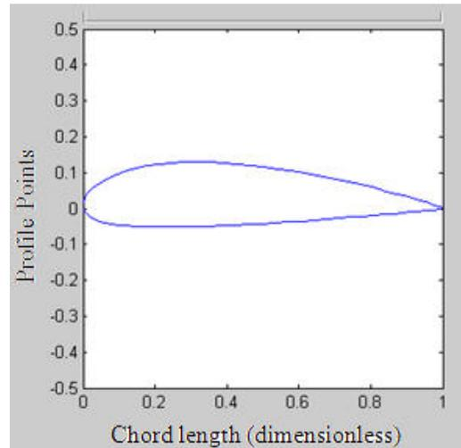
Figure 6. NACA 4420 profile, generated with MATLAB software.
