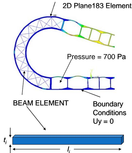
Figure 4. Topology design problem formulation and ground structure diagram.
