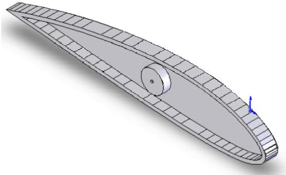
**Figure 18. Cover to seal the open end of the UAV wing.**
