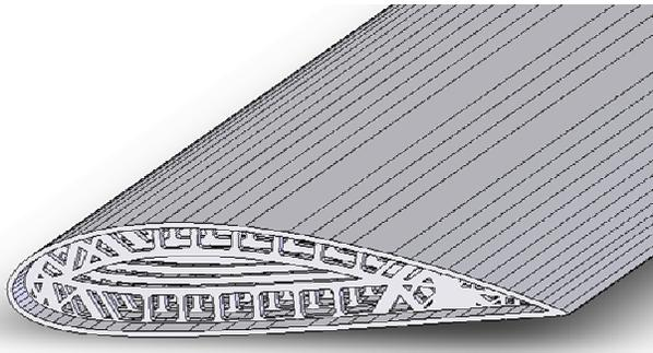
**Figure 16. Cross-section of 3D CAD model of UAV wing.**
