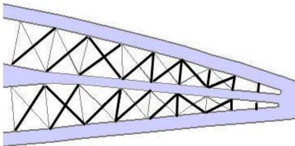
**Figure 13. UAV right section optimization showing retained lattice elements in bold.**
