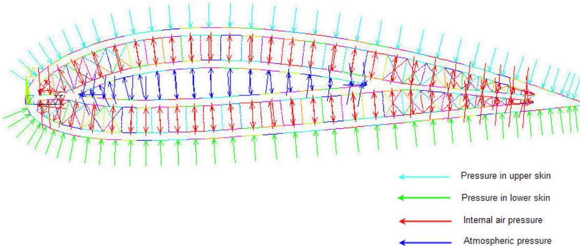
Figure 8. Pressure profile applied in ANSYS.
