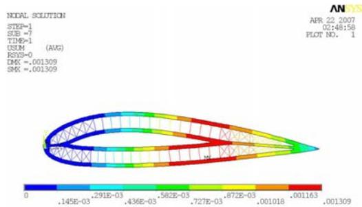
**Figure 14. Deflection result of UAV WING after right section optimization.**
