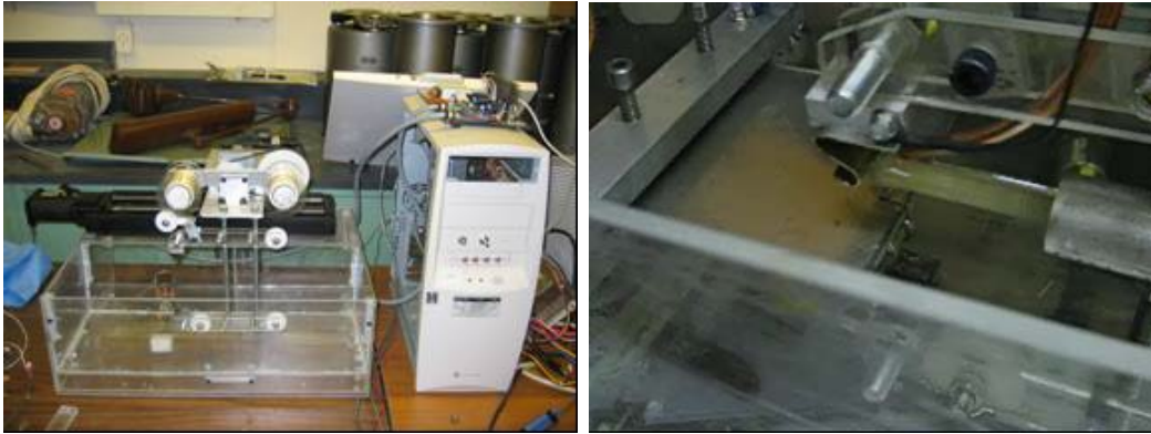
Figure 14. Realization of the wire-EDM machine: system oval (left) and cutting a titanium sample (right).
