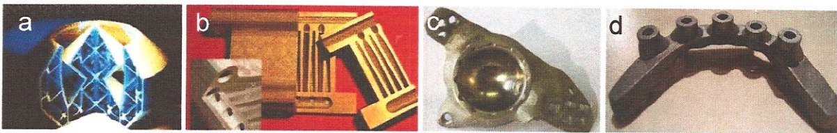
Figure 1. Sample parts produced by SLM: A hollow reinforced part made by Trumpf (a); A heat exchanger as satellite component made by K.U.Leuven (b); An acetabular hip implant cup made by Arcam (c); A dental framework for the support of dental implants made by K.U. Leuven (d).
