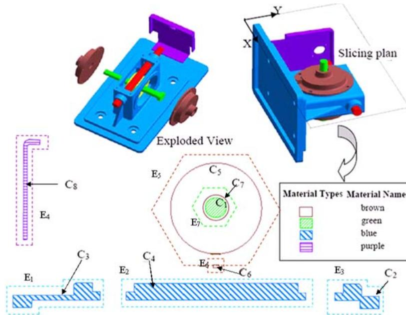
Figure 12 A CAD model a gearbox assembly and slice of it
