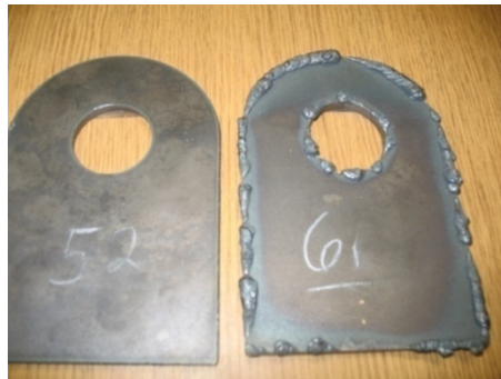
Figure 4. A Perfect Cut (Part 52) vs. a Part With Residuals (Part 61).
