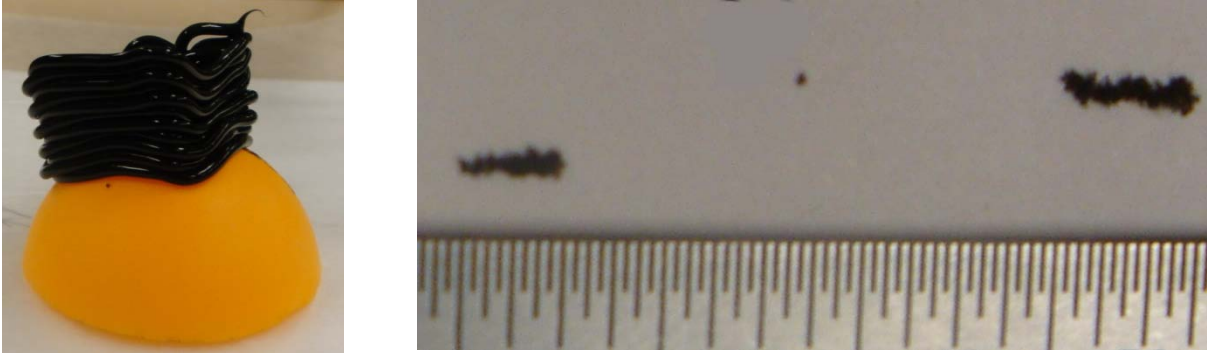
Figure 5: System test: (a) Complete structure test: A silicone-based caulking material was used to form a cube on top of an existing hemisphere; (b) Reliability Test: The hash marks are 1/64" apart.
