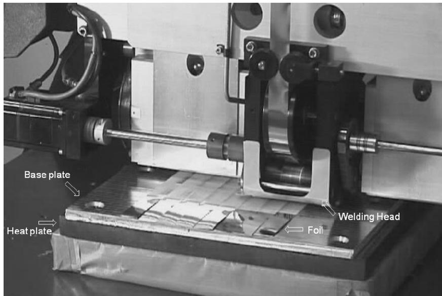
**Figure 5.** Base plate and part fixture in the Solidica Formation™ machine
