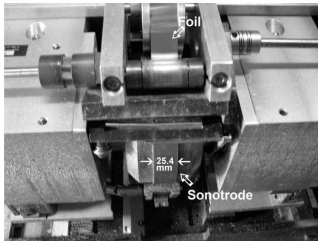
**Figure 3.** Close-up view of the Welding head, showing the sonotrode from below (as shown in [3])
