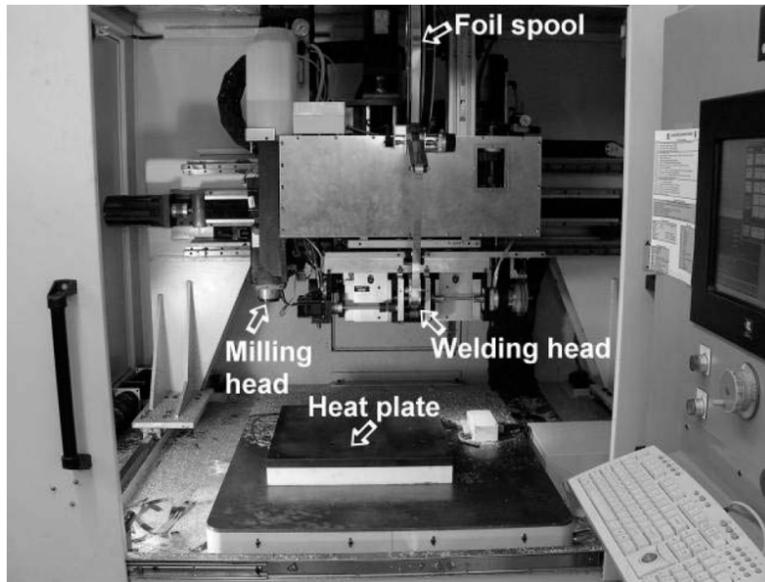
**Figure 2.** Solidica Formation™ machine (as shown in [3])
