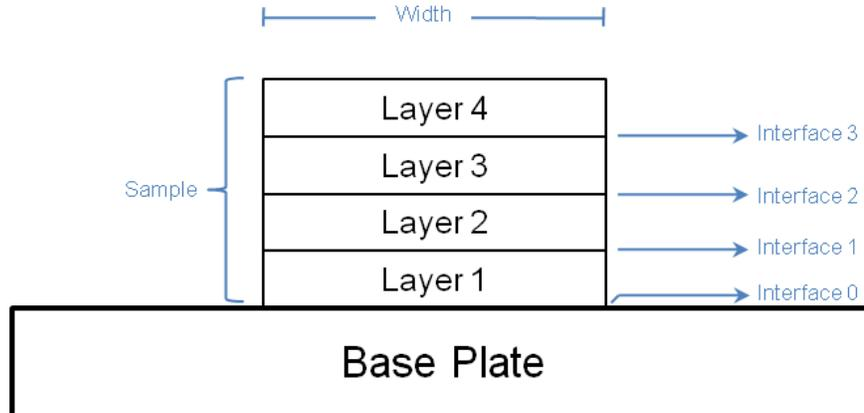
**Figure 9.** Sample welding interfaces
