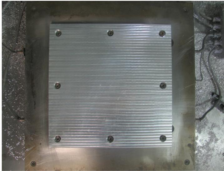
**Figure 4.** Geometry of the base plate used within the Solidica Formation™ machine and bolt locations just before deposition
