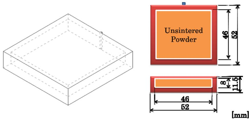
Fig. 4 Test specimen for packing density measurement
