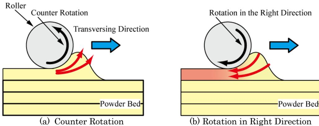
Fig. 1 Two types of roller operations
