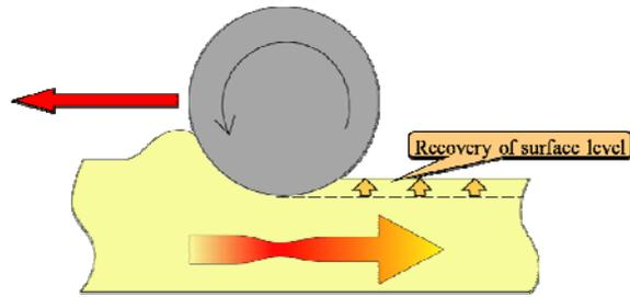
Fig. 11 Schematic view for compaction at high compaction factor
