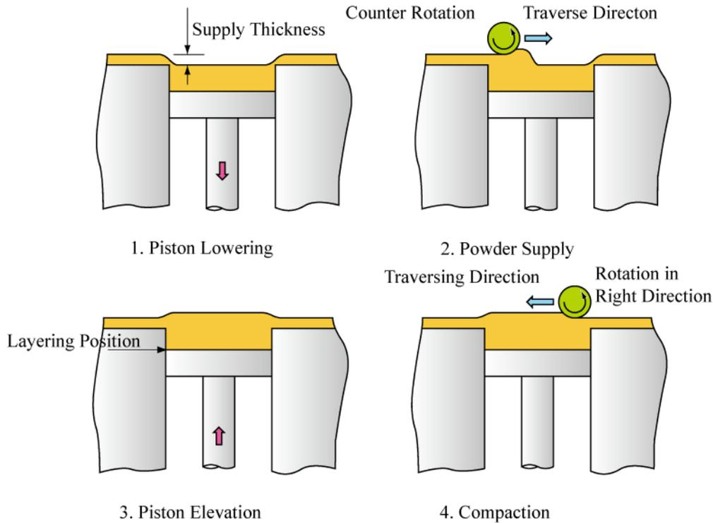
Fig. 3 Compacting Method
