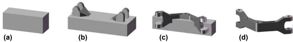
**Figure 1 – Multiple setups required (even in multi-axis milling) to create component via a subtractive process; (a) shows initial stock geometry and (b-d) show the results after iterative cutting operations until (d) the component fully emerges**
