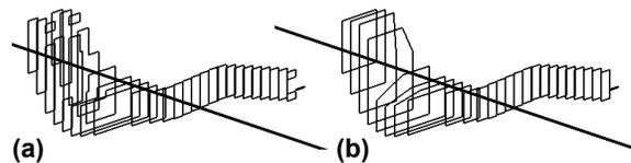
**Figure 6 – Each slice (a) is represented as (b) its convex hull polygon**
