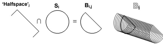
**Figure 9 -  $\mathbb{B}_j$  is the set of slices  $B_{i,j}$  composed of stock material unreachable from angle  $\alpha_j$  to depth  $\delta_j$ , computed by trimming the unreachable ‘halfspace’ to the stock cross-section**
