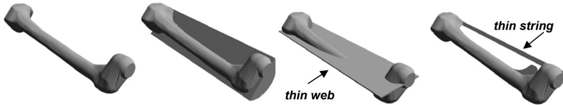
**Figure 13 – Examples of thin webs and strings emerging from the multi sided machining of a human femur from round stock**
