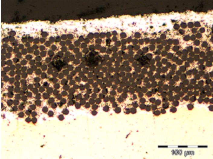
**b: Higher magnification of Cu/MetPreg on Al 3003-H14 substrate**
