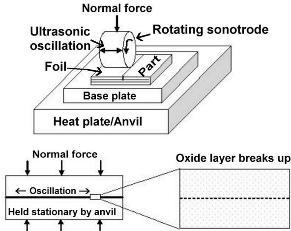
**Figure 1: Schematic of UC process**
