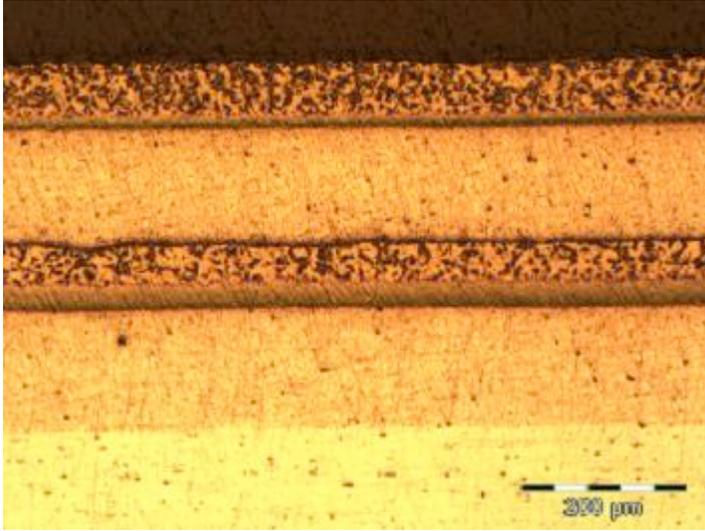
**b: Al 6061/Ti/Al 6061/Ti on Al 6061-T6 substrate**
