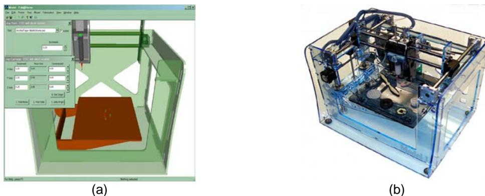
**Figure 2: Fab@Home Graphic User Interface (GUI) and Machine.** (a) Using the Fab@Home software platform, we were able to control the motion of the (b) gantry and deposition tools.
