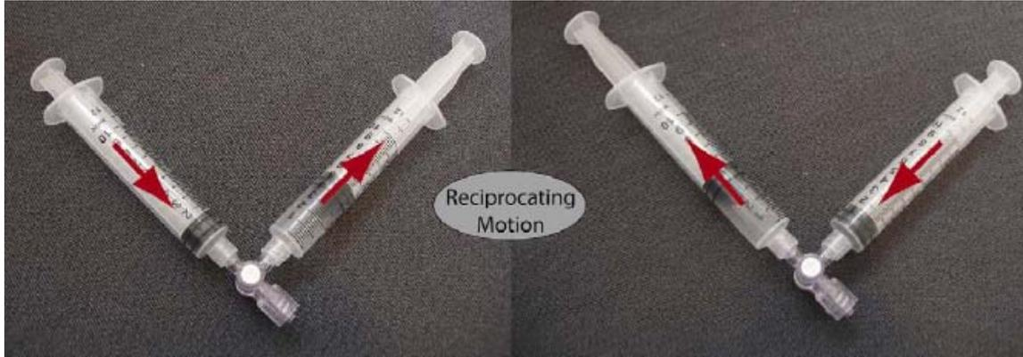
**Figure 1: Reciprocating Motion.** This reciprocating motion, adopted from Cohen *et al.* [14] was implemented to mix the 1% calcium sulfate with the 2% alginate solution to produce a single stiffness hydrogel.
