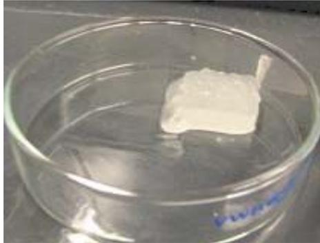
**Figure 4: Single Stiffness Hydrogel via Premixing.** A single stiffness, 1" by 1", alginate hydrogel cube made of 20 layers was successfully printed using the Fab@Home.
