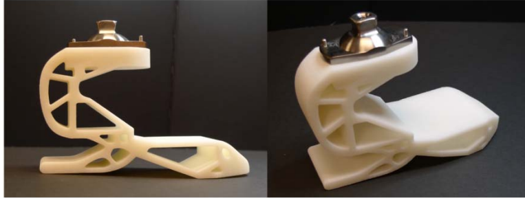
Figure 9. Final design prototype manufactured from Nylon-11 using SLS technology.
