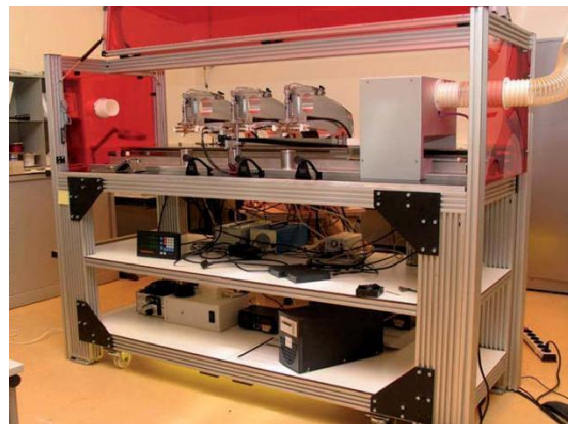
Figure 3 – The high viscosity inkjet printing test rig
