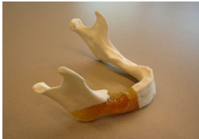
Figure 9- bioresin implant inserted into model of mandible
