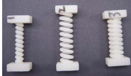
Figure 6: Three types of spring designs used in static testing
