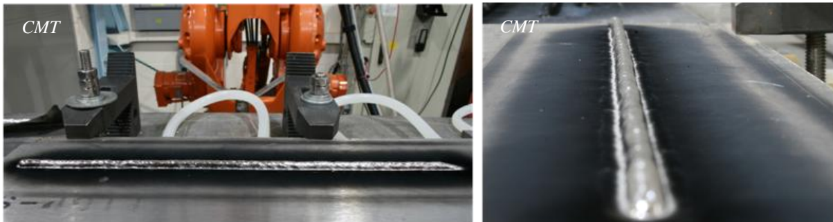
Fig. 4 CMT single bead on plate Ti-6Al-4V deposits showing that the cathode spot relocation mechanism was prevented and the spattering mechanism suppressed.
