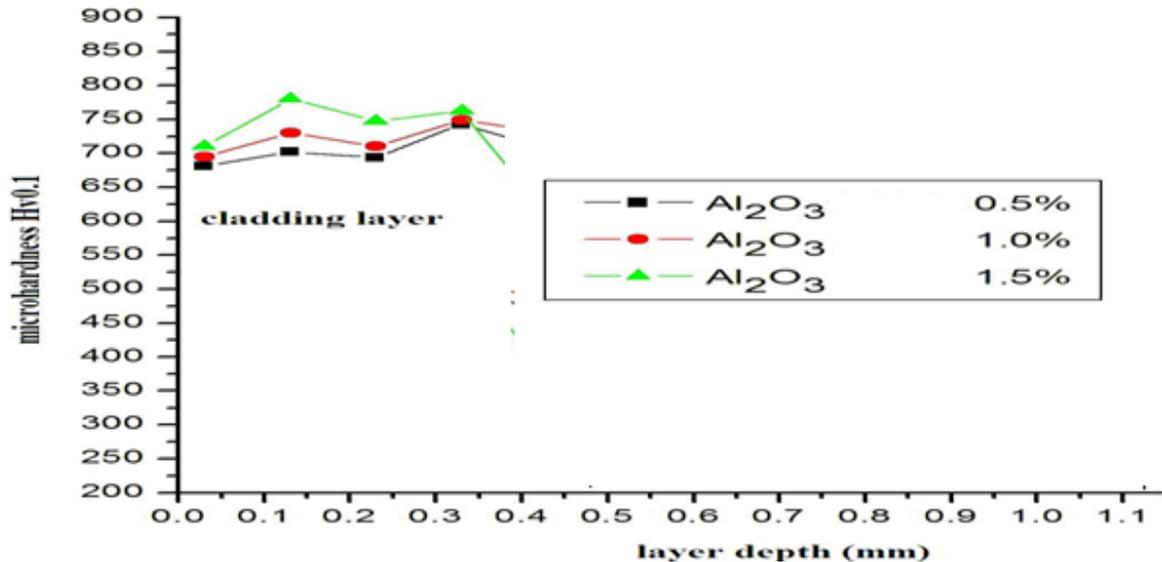
Fig. 8 micro hardness of cladding layer
