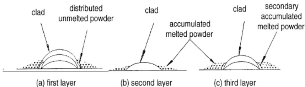
Fig 2 Layer cladding
