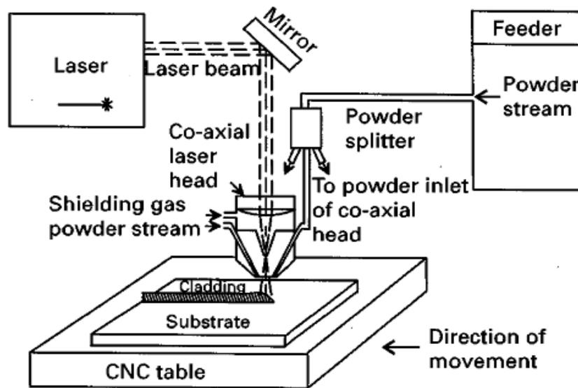
Fig. 1 CO<sub>2</sub> laser cladding schematic drawing
