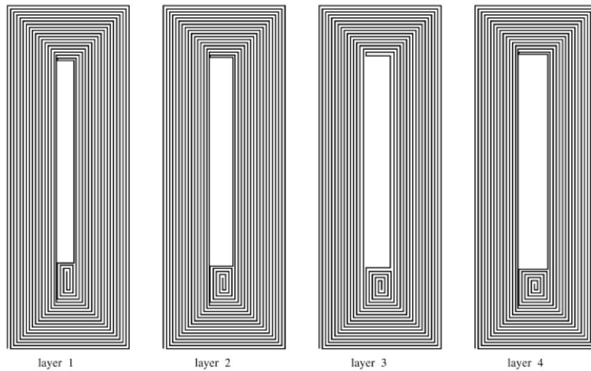
Fig. 4 Layer profile of the cladding path for the part.
