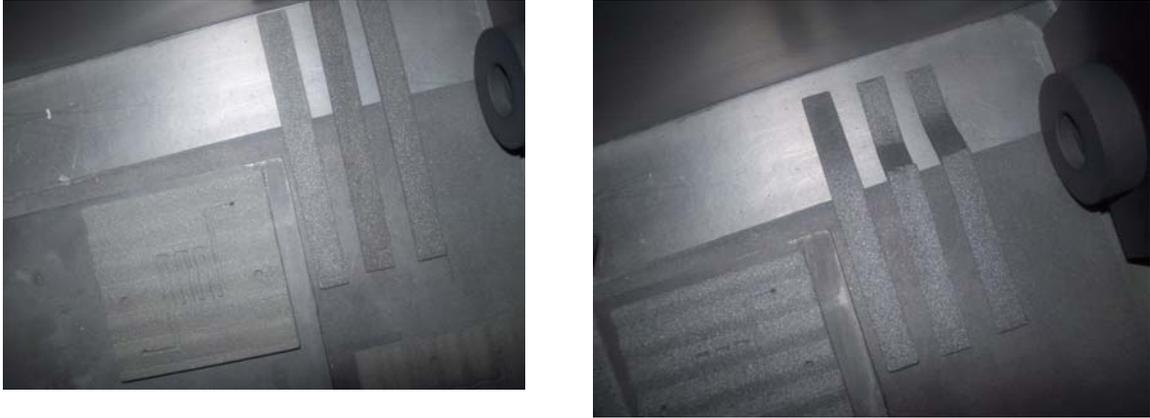
Figure 11: 3 point bend specimens in the furnace before and after vacuum furnace processing. All the parts were slumped after carbonization at 1200°C.
