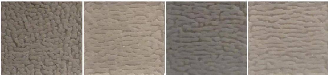
(c) Effect of Laser power (L-R: 15, 20, 22 and 25 W) at Scan speed = 50.8 mm/s and Scan spacing = 0.076 mm
