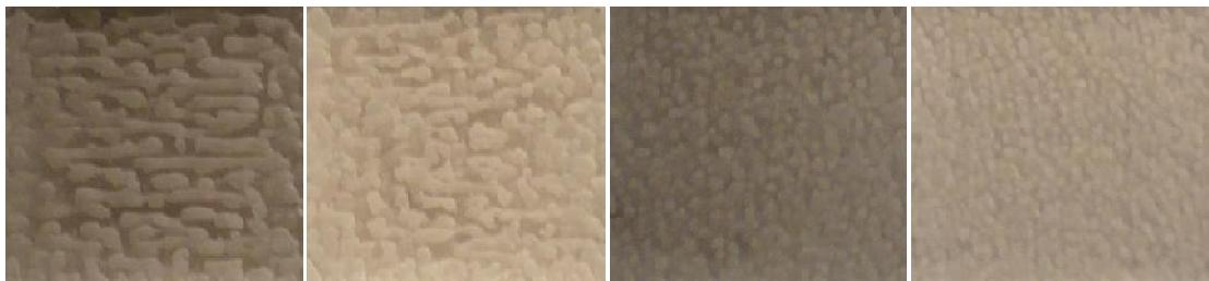
(a) Effect of Scan speed (L-R: 50.8, 76.2, 101.6 and 127 mm/s) at Laser power = 25W and Scan spacing = 0.076 mm
