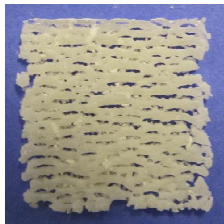
Figure 2. Mono layer laser sintered at 20W (25.4 mm x 25.4 mm)
