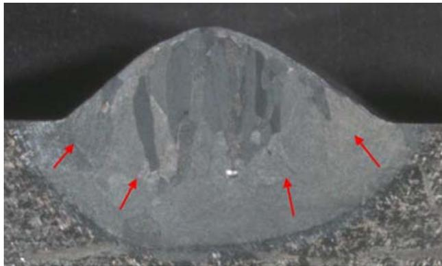
**Figure 4.** Cross section micrograph showing the deposited bead, the remelted substrate boundary (see arrows) and the substrate heat affected zone
