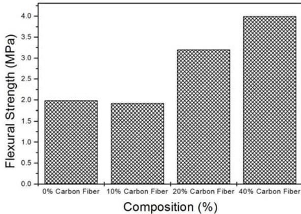
Figure 5 a) Flexural strength of green parts w.r.t addition of carbon fiber.
