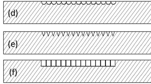
Figure 4 d) elliptical, e) triangular and f) rectangular flow fields with 15 passes.
