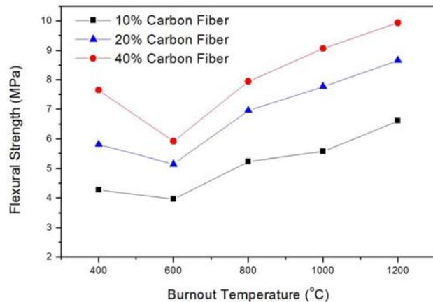
Figure 5 b) Flexural strength of brown parts w.r.t burnout temperature.
