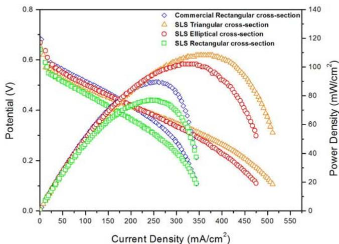
**Figure 7 c) DMFC polarization curves of 5 cm<sup>2</sup> flow field area bipolar plates (15 passes)**
