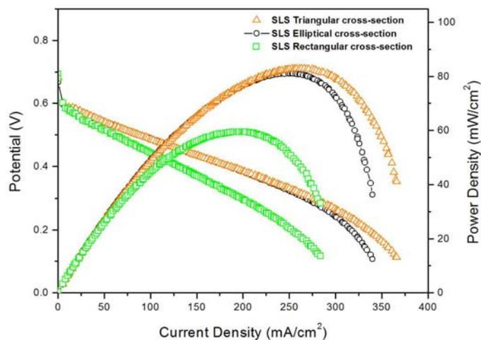
**Figure 7 b) DMFC polarization curves of 10 cm<sup>2</sup> flow field area bipolar plates (10 passes)**
