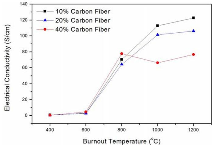
Figure 6 b) Electrical conductivity of carbon fiber added parts w.r.t burnout temperature.
