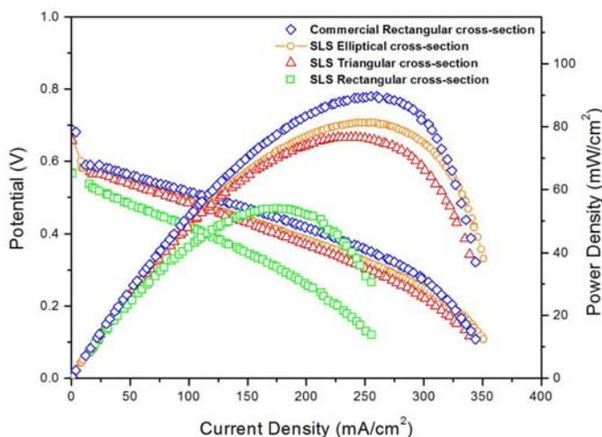
**Figure 7 a) DMFC polarization curves of 5 cm<sup>2</sup> flow field area bipolar plates (10 passes)**
