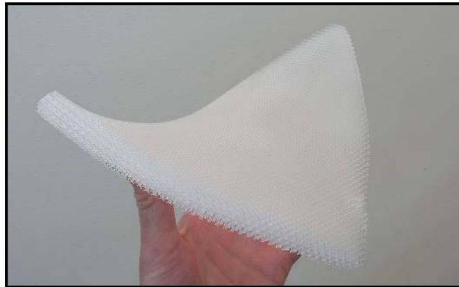
Figure 5. Example of a micro-lattice structure with anticlastic curvature.
